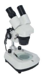
Our versatile 10x/30x stereo microscope features three-way LED illumination (top, bottom, or both), paired 10x WF eyepieces, and 1x/3x objectives on a rotatable turret. The head is rotatable 360° and can be rotated on its mounting pole to view objects too large for the stage. Includes a frosted glass stage plate, reversible black/white stage plate, two metal stage clips, and a vinyl dust cover.
