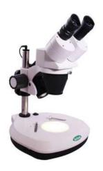
Our Stereo Microscopes features precision optics to ensure the highest level of performance for inspection and dissection. All models also come with upper and lower LED illumination to provide the brightest and most energy-efficient lighting available on the market.
